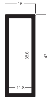
Z 100 Beam extrusion 43 mm 3.14 kg | 5000 mm
